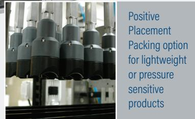
Positive Placement Packing option for lightweight or pressure sensitive products
